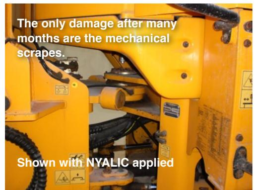
The only damage after many months are the mechanical scrapes.
